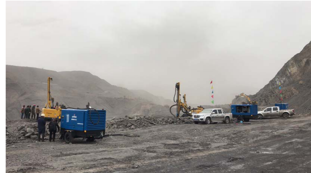
Blasting drilling in coal mining (3xLUY180-19 plus DTH rig each)
